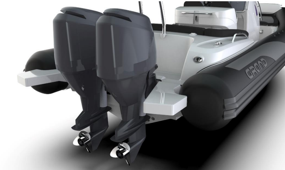
Fig. 53. Twin engine installation.
